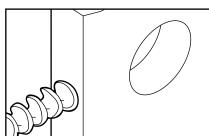
Drill a 25mm hole in the centre of the door edge through to the 54mm hole.
