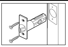
**3.** Insert the latch and tighten the screws.
