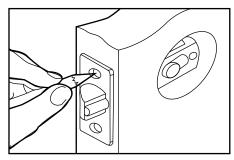
1. Insert latch in hole. Keeping it parallel to door face, mark outline of latch face and screw holes. Remove the latch.
