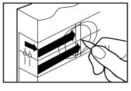
Mark the centre point of the lockset hole on the door face at the desired backset, either 60mm or 70mm.
