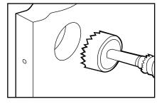
Using a 54mm hole saw, drill through the face of door. It is recommended that holes be drilled from both sides to prevent splitting.
